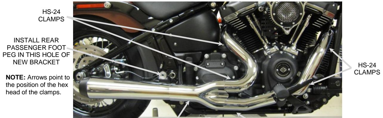
FIGURE 4 SPECIAL NOTE: FIGURE ABOVE SHOWS STREET BOB WITH MID CONTROLS. FAT BOB IS THE SAME ONLY WITH FORWARD CONTROLS.
